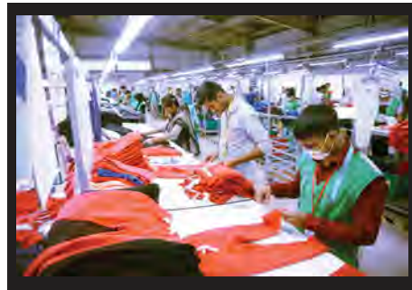
Finished Fabric Inspection
